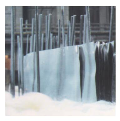
Soonv ® G-30® alloy has outstanding resistance to hydrofluoric/nitric acid mixtures such as employed in the pickling of stainless steel. This particular operation involves aerated, 15% HNO<sub>3</sub> and 5% HF at 140 deg. F. (60 deg. C)
