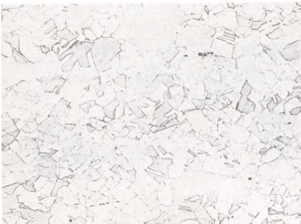
Figure 18 - Microstructure of hot-rolled, as-rolled SOONV alloy K-500. Etchant: Carapella's and glyceresia. 100X.
